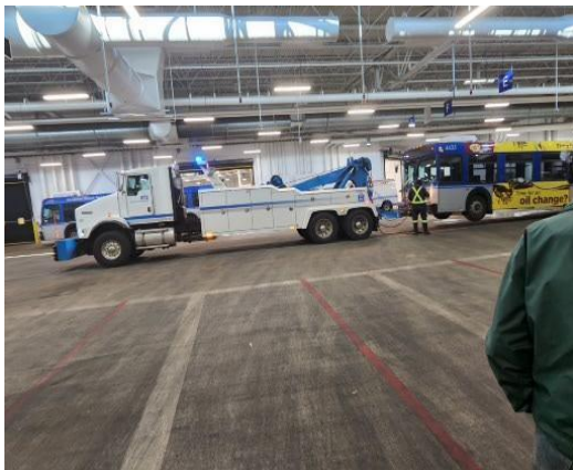
A tow vehicle halling a "dead" bus. In this picture he is decoupling it. It will be taken from here into the garage for repair.
