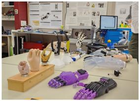
Here we have range of devices that were developed or acquired to research artificial hands. Researchers are particularly interest in understanding how to enhance sensory feedback. The ones on display are designed to provide sensory feedback with out surgery. Such as surgery which attaches artificial limbs to existing nerve ends.
