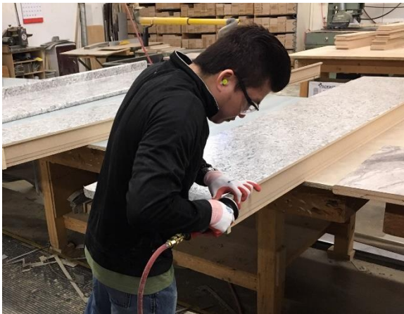
A worker in the laminated countertop production area finishes the edges on a kitchen countertop.
